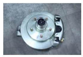
To check your bearings, raise your wheel clear of the road surface (by the procedure indicated in "tire changing"). With your hands on the outside edges of the tire, try to rock the wheel by pushing on one side and pulling on the other. No noticeable rocking should occur. Spin the wheel and listen for noise or roughness. A smooth, silent operation means that your bearings are in good order. If a grinding sound is heard, contact your SKEETER Dealer for warranty and or replacement instructions.
